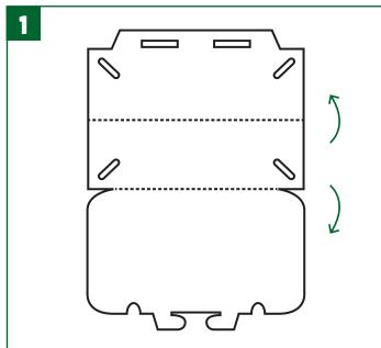
Remove all six perforated slot openings then fold creases inwards and insert bottom tabs into top slot.
